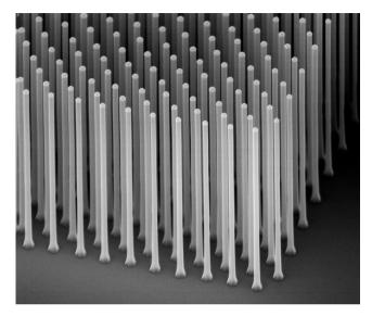
A regular array of nanowires, grown from seed particles (still visible on top of the wires) that were positioned on the substrate using nanofabrication techniques. The diameter of the wires is about 100 nanometres, more than a hundred times thinner than a human hair.
